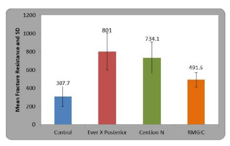
By using one way ANOVA statistically significant variation was found in mean fracture resistance in samples of four groups (F=23.37,p=0.0001).
