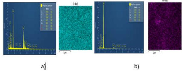
Fig.13. EDS spectra a)dispersion with UPW, b) dispersion with solvent
