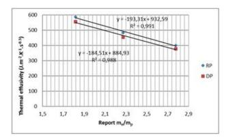
Figure 9. Eco-plaster thermal effusivity according to mixing rate
