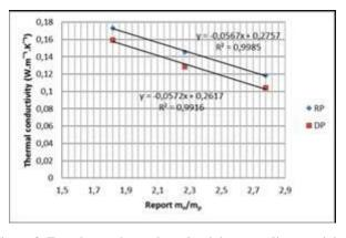
Figure 8. Eco-plaster thermal conductivity according to mixing rate
