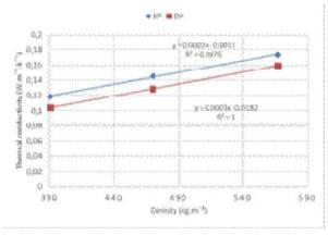
Figure 7. Thermal conductivity variation according to density
