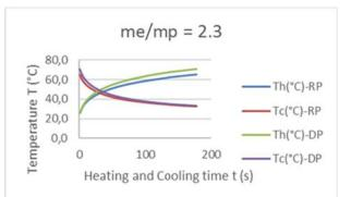
Figure 10-b. Plaster samples heating and cooling thermograms  $\frac{m_e}{m_p} = 2.3$
