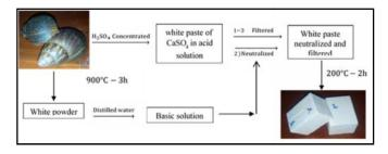
Figure 2. Eco-plaster synthesis from snail shells
