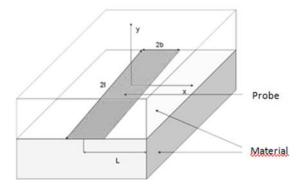
Figure 5. 2D model hot strip
