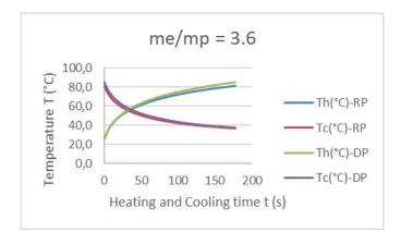
Figure 10-d. Plaster samples heating and cooling thermograms  $\frac{m_e}{m_p} = 3.6$
