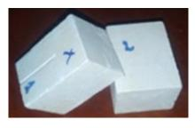
Figure 3. Plaster specimens
