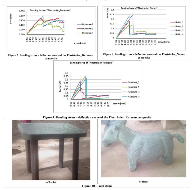
The making of the Horse (see photo 19 below) required about 12 kg of resins (PP) and 3 kg of reinforcements (short duramen fibres), i.e. 15 kg of the "PLASTRONIER" to be cast. These two objects, which are useful for childcare centres, required a total of 25 kgs of plastic waste and 6 kgs of reinforcements from the tall-palm tree. For a production of 1000 items, 25 tonnes of plastic waste will have been eliminated from the environment.
