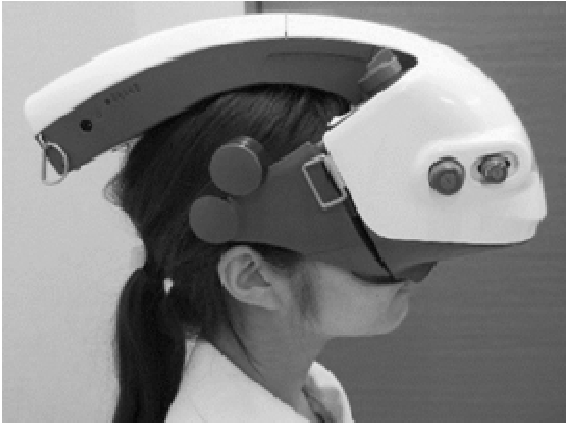
Figure 1. Head-mounted imo perimeter weighing 1.8 kg
