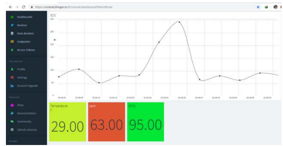
Figure (3.1): Photo showing the results from thinger platform
