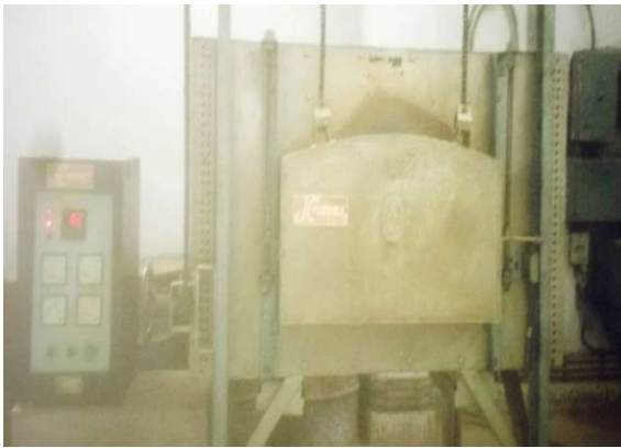
Figure4 Muffle Furnace: Both the collected metal and slag samples were analyzed. Optical emission spectrometer (ARL 3460) was used for analyzing metal samples whereas slag samples were analyzed using (XRF PW 2400). The metal samples were taken out from metal mould and the surface on which the sparks were to be made was machined. Metal samples were polished using aluminium oxide paper 60 grade To ensure homogeneity sparking were carried out at four different points in Ar atmosphere. and then the average result was taken.
