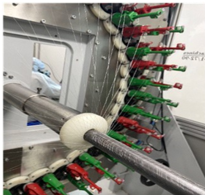
(B) The fibers are transformed into yarn, which serves as a medium for the subsequent braiding process.
