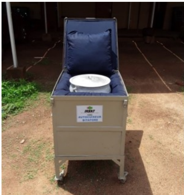
Figure 2. Prototype of a metal model pressure cooker
