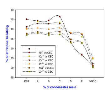
The order of CEC of the resins and condensates for the exchange of divalent metal ions is of the order:  $Ni^{2+} > Cu^{2+} > Ca^{2+} > Pb^{2+} > Mg^{2+} > Zn^{2+}$  This may be due to the selectivity of the metal ions for ion exchanger process. From the results given in table V (Fig. 4), it is noted that condensates upto 30%
