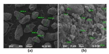
Fig.4 showed the SEMs of before and after metal ion removal. However, the particles of (Fig.4a) had a rough surface with heterogeneous holes and pores that make a large surface area, which indicated that metals can be adsorbed onto its surface. Fig.4b showed micrographs of the NNSC surface after adsorbed metal ions, the surface of NNSC was relatively smoother and less porous because of the formation of a layer over the adsorbent surface after adsorption of metal ions.
