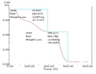
Fig.3.TGA for 30% condensate resin
