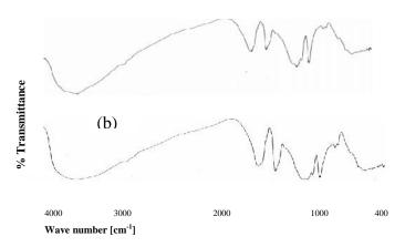
Fig. 1 FT-IR Spectra of PFR, (b) PFR blended with 30 % (w/w) NNSC in composite
