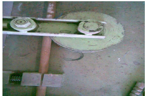
Fig. 2. Bending roll and fixture with tube
