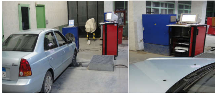
Fig. 1 Experimental equipment used during dynamometer testing
