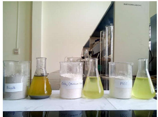
Fig.7. Precipitation of Barite is clearly shown after 30 minutes of reaction with HCl
