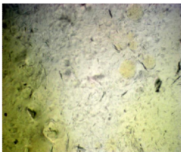
c- Fuel oil + 2000 ppm, C_{14}E_{14} , PP = -3°C, CP = 20 °C
