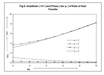
The amplitude and phase of heat transfer in shown in Fig. 9. It is observed that amplitude of heat transfer increases with increasing  $\omega$  for small value of Re (i.e. increase in frequency of oscillation generate more heat due to increase in velocity of fluid hence more transfer of heat to the plate) and than
