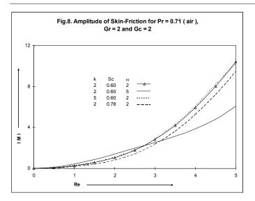
It is observed that phase of skin friction increases with Gc while reverse effect is observed for Gr. There is always a phase lead with increasing  $\omega$ . The magnitude of phase of skin friction in lower in case of Sc=0.78 (NH<sub>3</sub>) than that of Sc=0.60 (CO<sub>2</sub>). We now study the effect of various parameters on the rate of heat transfer. The rate of heat transfer in terms of the Nusselt number at the plate can be obtained as
